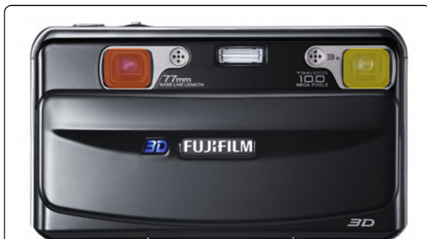
Figure 1 Illustration of a multispectral-stereo system constructed from Fujifilm 3D camera and a pair of filters placed on top of the two lenses.
