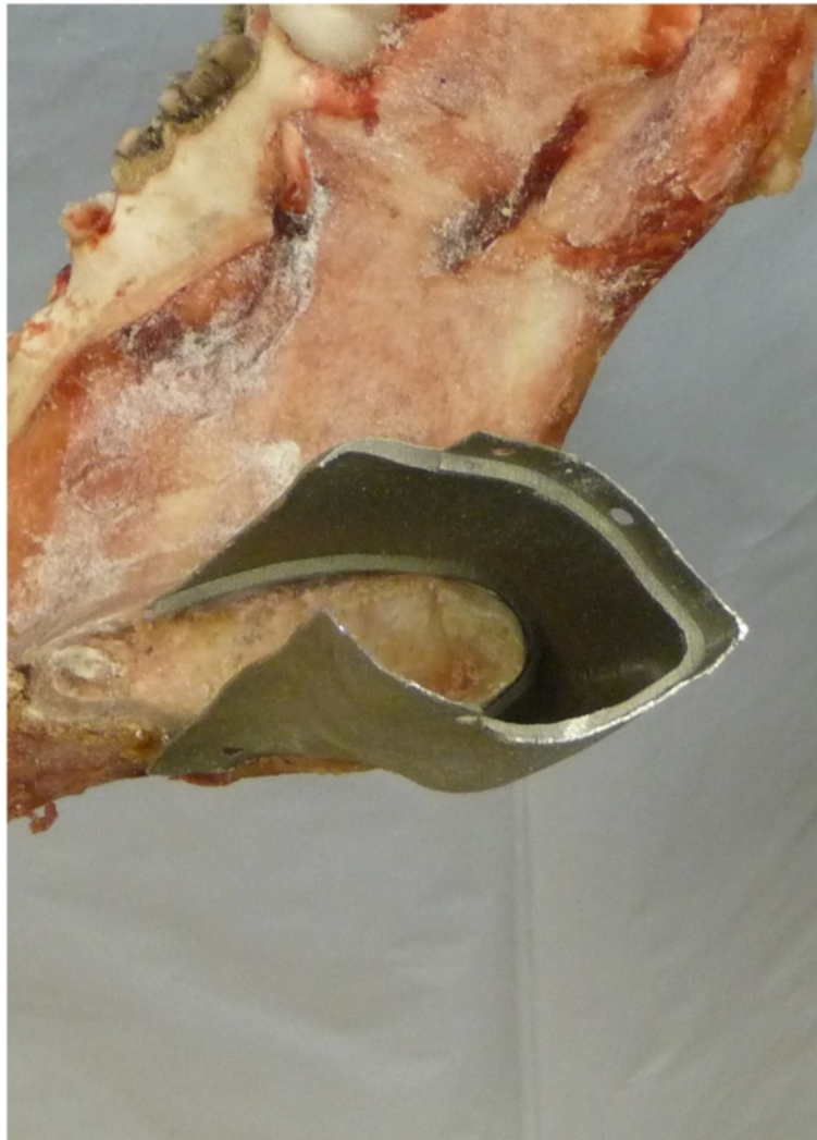
Fig. 5 Detailed view into the connection area of the bone – implant area. A tight fit was achieved between all implants and the bone
