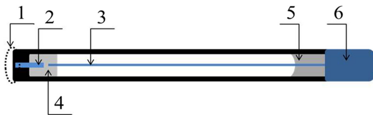
Fig. 2 Scheme of platinum disc electrodes. 1 Bioselective membrane, 2 platinum wire, 3 inner conductor, 4 wood alloy, 5 epoxy resin, and 6 contact panel
