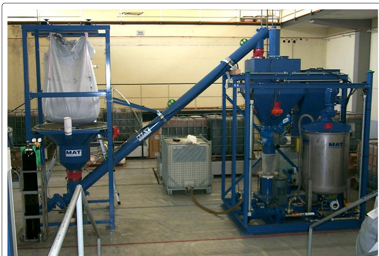
Figure 21 Continuous 1-t/h bioslurry preparation with colloid mixer.
