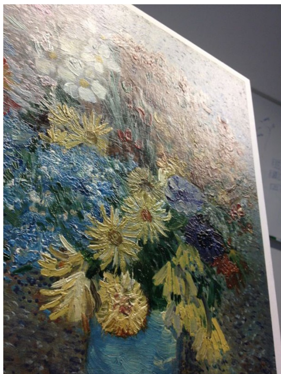
Figure 7 The 3-D printed van Gogh painting. The reflection of the raking light enhances our perception of the brush strokes. This particular print was made on foam board, which was later framed.
