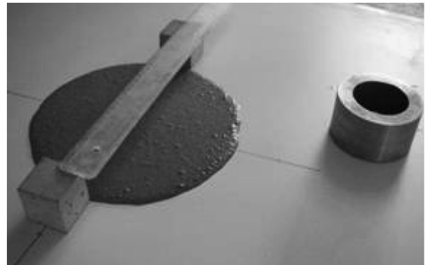
Fig. 3 Mini-slump test for fresh FSC.
