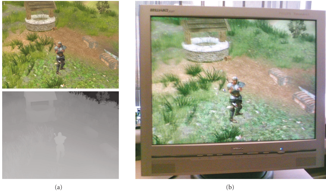
FIGURE 14: Screen shot of GOAL: image and depth buffers (a), and actual image on autostereoscopic 3D display (b).
