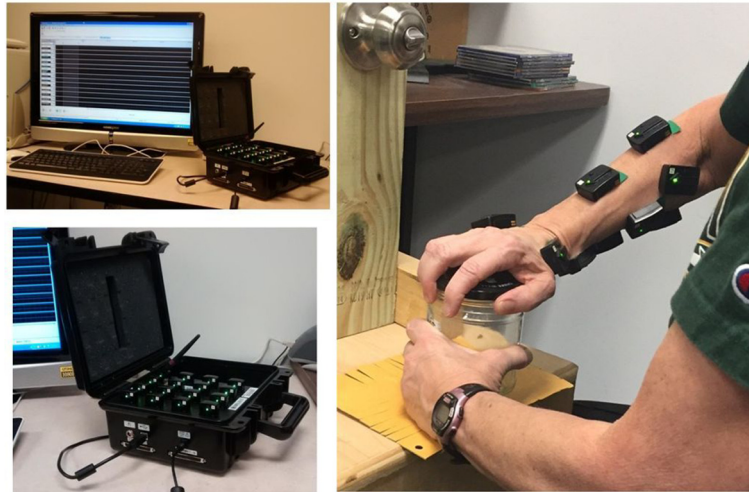
Fig. 1 Trigno kit used for data collection (left, top and bottom) and a subject (right) performing a jar lid turn with ten sensors attached to the action arm
