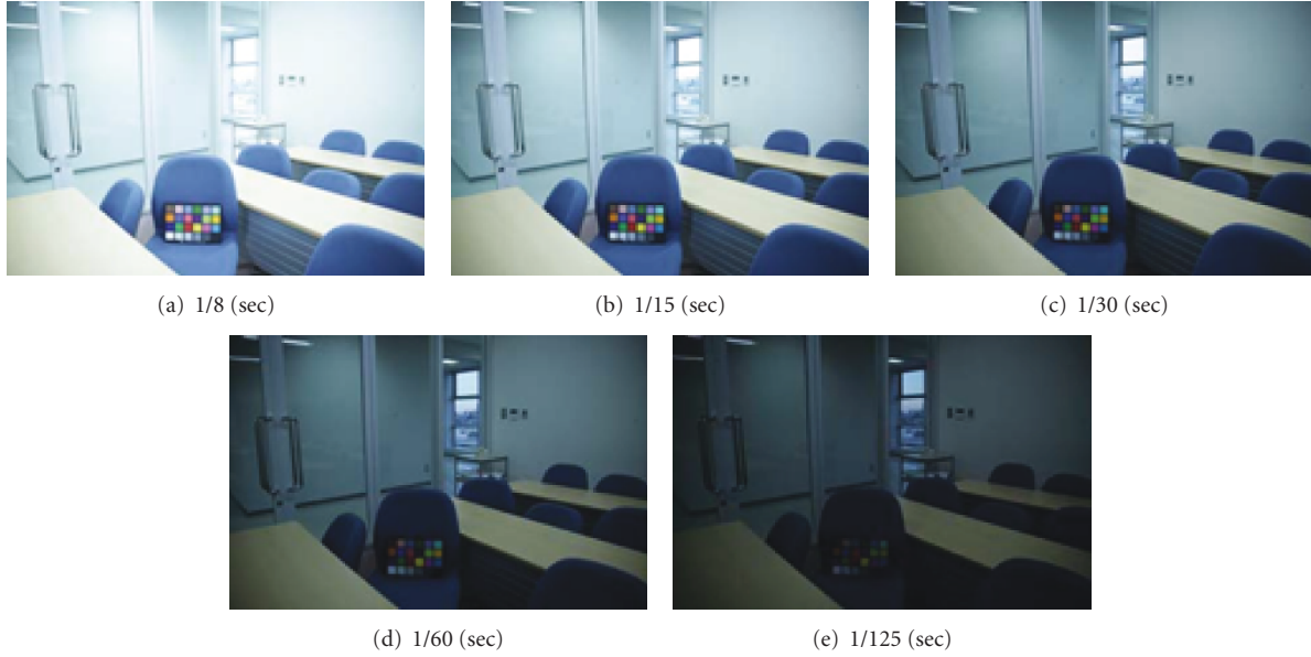
FIGURE 7: Camera images captured with different exposure times for the scene “Meeting Room.”
