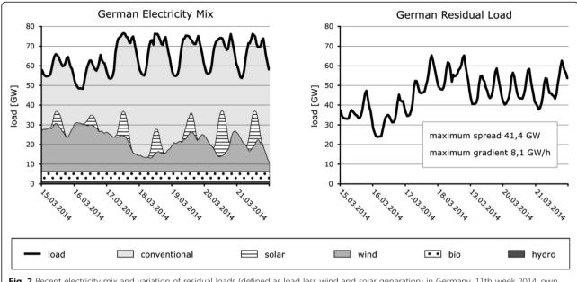
Fig. 2 Recent electricity mix and variation of residual loads (defined as load less wind and solar generation) in Germany, 11th week 2014, own presentation based on [102, 103, 104]
