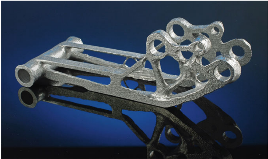
Fig. 5.14 Final light-weight part manufactured by SLM
