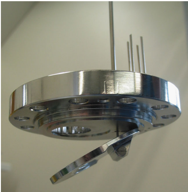
Fig. 2 Photograph of the open UCN flap valve. The vertical hole for UCN extraction can be closed by pulling the flap disk to the flange via a vertical actuator rod connected to a horizontal axis embedded in the disk, about which it is free to rotate. The flange is sealed with indium to the “T” section of the converter vessel (see Fig. 1)
