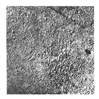
gas is used, the pores are smaller and appear to be distributed throughout the casting. Under full vacuum, no pores are found, but a new phenomenon in the form of increased surface roughness is noted which was related to the dendritic structure of the cast metal. Ott posed the interesting question whether the gas pores in a casting do possibly not contribute to the smoothness of the surface by compensating for the shrinkage of the solidifying metal.
