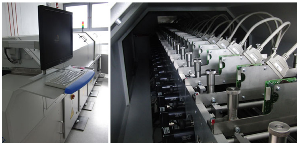
Fig. 2 Pictures of the latest laser printer generation: The 24 linearly aligned printing cartridges ( right ) in the printing track form the core of the 5.5 m long device ( left )
