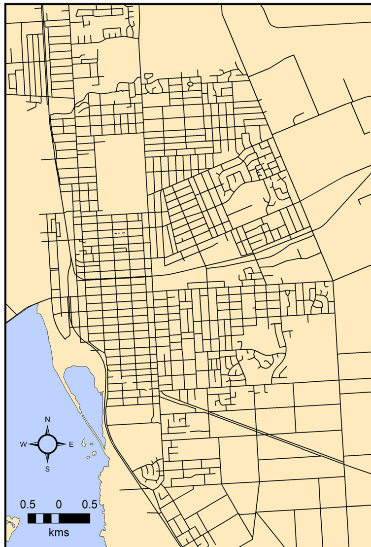
Fig. 3 The road pattern for urban Invercargill is largely based on a grid (data obtained with permission from Land Information New Zealand ( https://data.linz.govt.nz/ )). Rotations of L_1 will capture an approximate network road distance and the orientations of road sections
