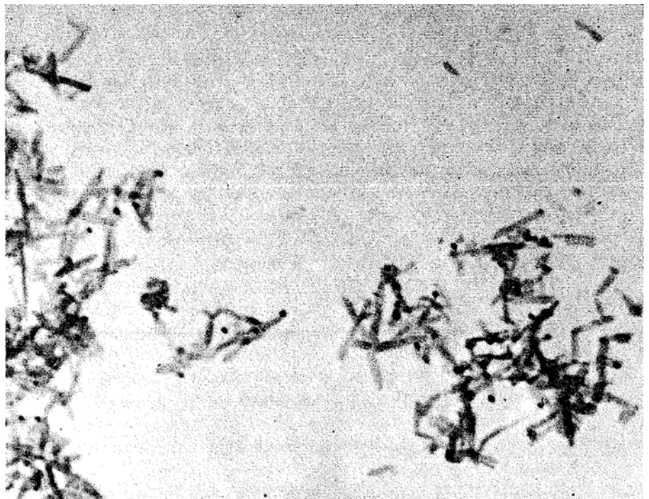
Fig. 15 Electron micrograph of 20% gold- 80% platinum catalyst adsorbed on alumina plates. x 300 000
