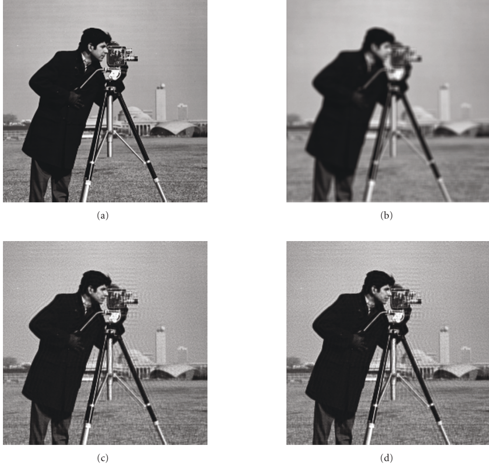
FIGURE 1: “Cameraman” image: (a) original image; (b) noisy-blurred image: PFS 5 \times 5 uniform box-car, BSNR = 40 dB; (c) restored image by LR corresponding maximum SNR in 355 iterations; (d) restored image by AALR corresponding maximum SNR in 200 iterations.
