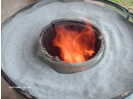
Fig. 2 The incinerator charged with red hot charcoal.
