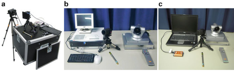
Fig. 22.6 (a) Rack mount type; (b) Desktop PC type; (c) laptop PC type of External appearance of IMES
