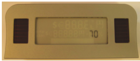
FIGURE 2: Photo of a fully functional energy harvesting electronic shelf label. This label has updated the price (70). We also see the two solar cells on this prototype.
