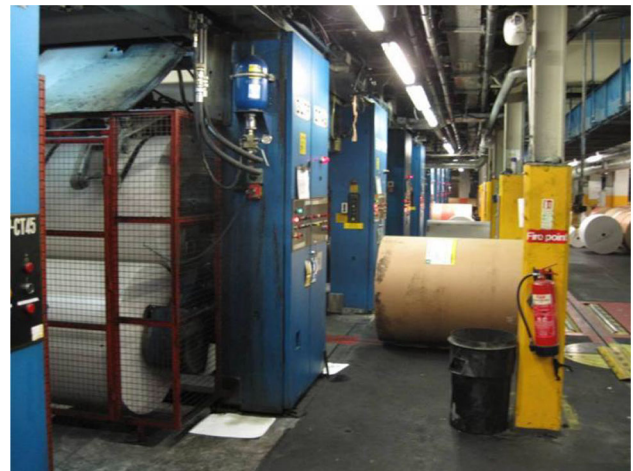
Fig. 4 Acoustically open reel stand where the operator exposure is 86 dB L_{EP,d}
