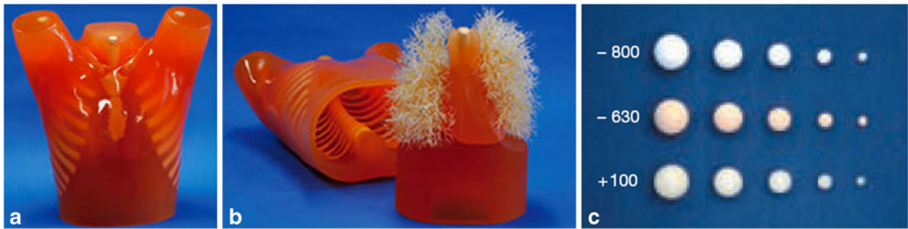
Fig. 1 a and b An anthropomorphic thoracic phantom with (c) artificial pulmonary nodules with five different diameters (3, 5, 8, 10 and 12 mm, corresponding to volumes of 14, 65, 268, 523 and 904 mm 3 ) and three different densities (-800, -630 and +100 HU)
