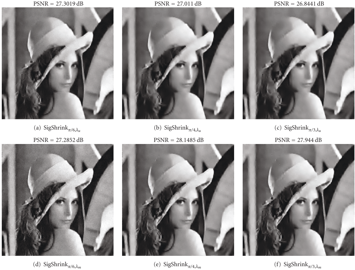
FIGURE 4: SWT SigShrink denoising of “Lena” image corrupted by AWGN with standard deviation \sigma = 35 . The universal threshold \lambda_u and the minimax threshold \lambda_m are used. The universal threshold (the larger threshold) yields a smoother denoising, whereas the minimax threshold leads to better preservation of the textural information contained in the image.
