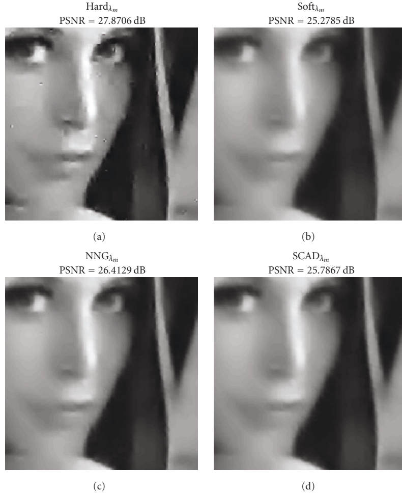
FIGURE 6: Denoising examples by using standard thresholding functions. The “Haar” wavelet and 4 decomposition levels are used for the wavelet representation (SWT). The denoising concerns the image of Figure 3.
