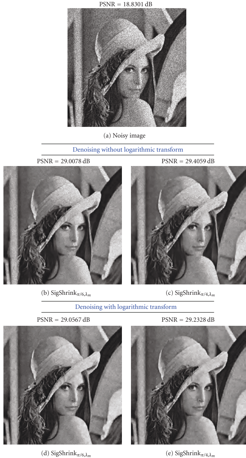
FIGURE 7: SigShrink denoising of the “Lena” image corrupted by speckle noise. The SWT with four resolution levels and the Haar filters are used. The noise standard deviation is estimated by the MAD normalized by the constant 0.6745 (see [4]).
