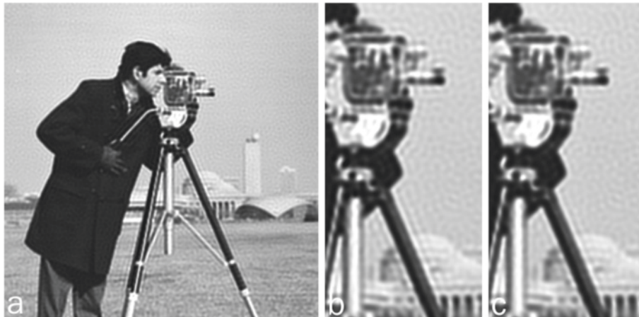
Fig. 19 Acceleration comparison. a Deblurred image by the accelerated RL method in [7], obtained at the 41st iteration with RSE = 0.54\% , b a zoomed part of (a) , and c a zoomed part of Fig. 9a, obtained by interlaced BI-RL with 4 \times 4 rectangularly-down-sampled blocks at the 26th iteration with RSE = 0.52\%
