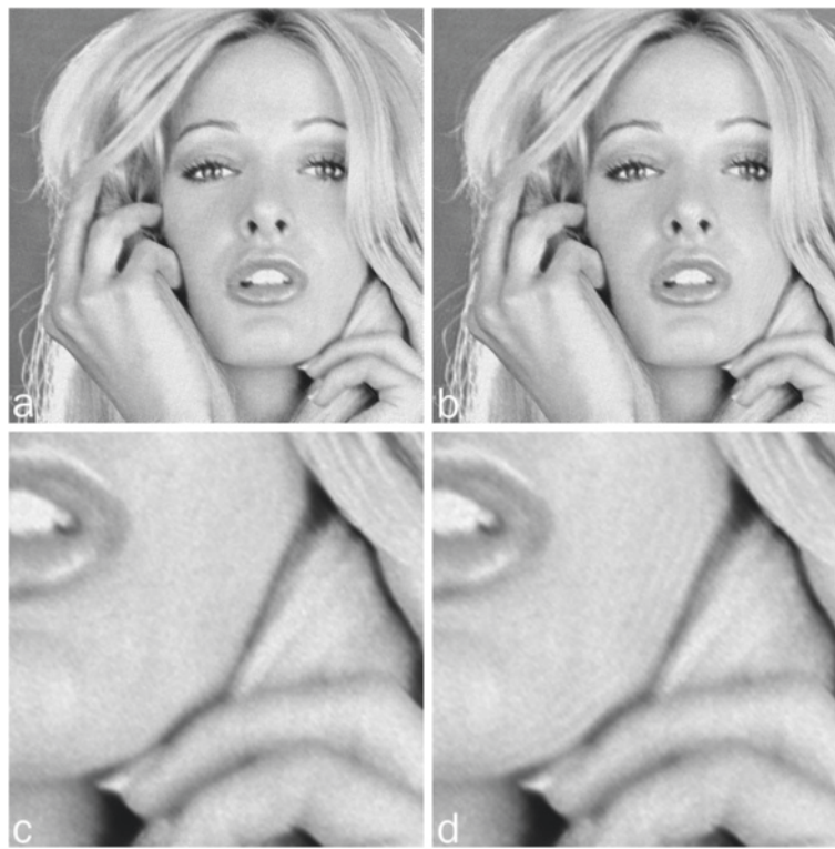
Fig. 11 Deblurred images by interleaved BI-RL with diagonally-down-sampled blocks and their zoomed parts. a 4 and b 8 diagonally-down-sampled blocks, c a zoomed part of (a) and d a zoomed part of (b) . These images were obtained at the 26th iteration with RSE = 0.65 % for (a) and 12th iteration with RSE = 0.67 % for (b)
