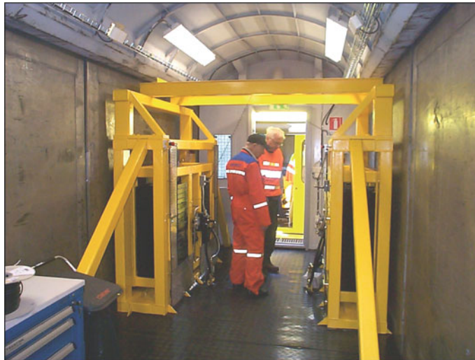
Fig. 2 Inside the RSMV, the weights in the rack above the rear axle are set in motion with hydraulic pistons [24]
