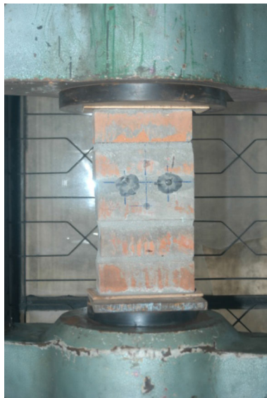
Fig. 1 Experimental set-up for static test (Brick masonry prisms)
