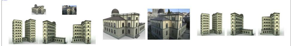
By including self-similar volume shapes, facade ornaments, repetitions and self-occlusion on a small scale, the Sternwarte is a very interesting example to model with the CityEngine [27]. Moreover, as the bottom row of Figure 4 shows, the facade design adapts to arbitrary variations of the underlying mass model. It would be easy to generate multiple models, if it would e.g., no longer be known how many storeys the building originally had, for instance.
