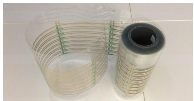
Fig. 4 Processed continuous and mass customizable R2R printed wiring board for flexible large area LED lighting system. Wiring board sample length 50 m, roll width 300 mm, wiring area total width 190 mm, substrate thickness 125 \mu\text{m} , printed conductive trace thickness 13 \mu\text{m}
