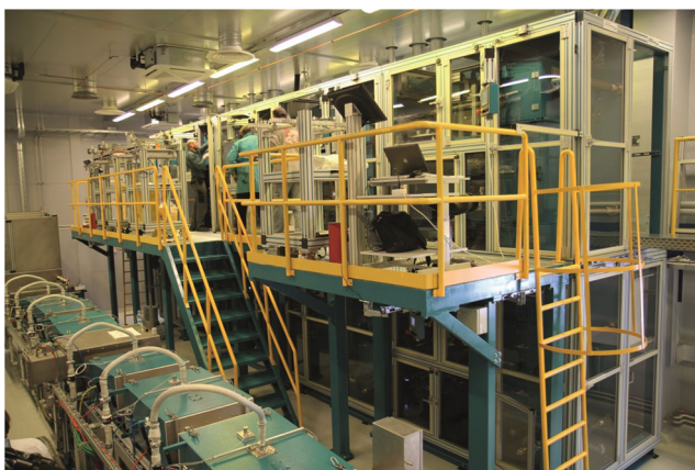
Fig. 3 MAXI roll-to-roll pilot printing machine used in the printing of the conductive traces on continuous and mass customizable LED lighting foil substrate
