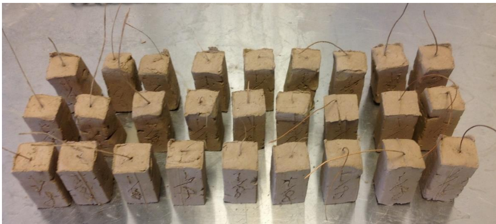
Fig. 4: Drying samples for pull-out test
