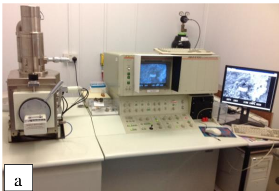
Fig. 5: Analysing Specimens for Gaps with (a) JSM-6100 Scanning Microscope, (b) OLYMPUS BX40 Computerised Optical Microscope
