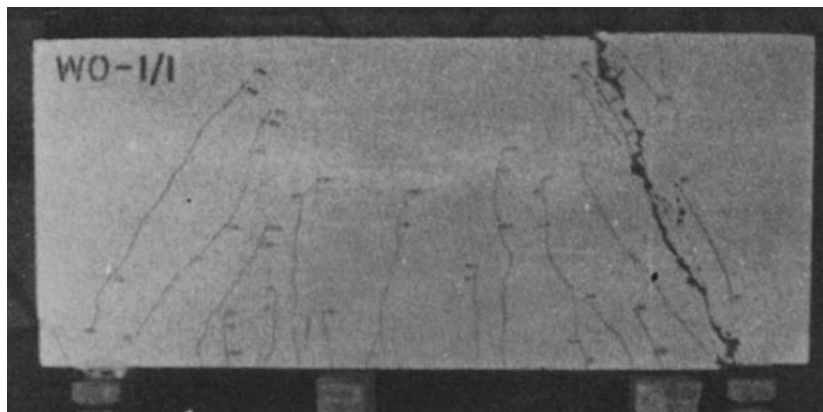
Figure 2.7 Failure mode of control specimen by Mansur and Alwist (1984)
