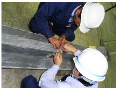
Fig. 6 Optical fiber sensor installation on the specimen.
