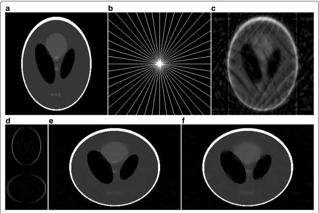
**Fig. 4 a** Shepp-Logan Phantom image. **b** 22 sampled radial lines. **c** Noisy image with a SNR of 20 dB. **d** Location of non-zero elements in the difference map. **e** Recovery image using CSMP with s = 4000 and q = 50 and only using 22 radial lines. **f** Recovery image using GAP and only using 22 radial lines
