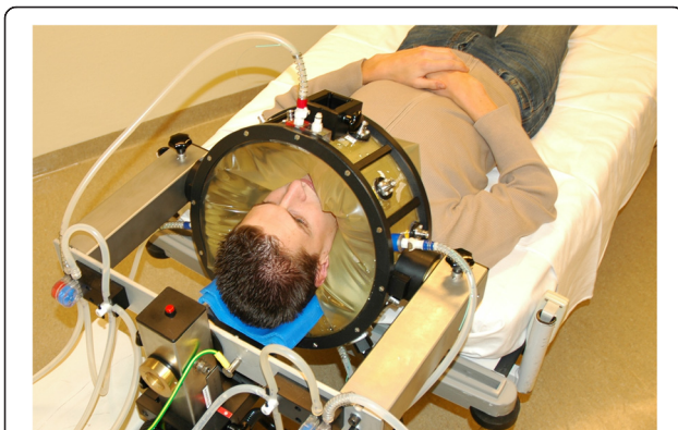
Fig. 1 The HYPERcollar applicator, as it was used until 2014, surrounding the 1 st author. This applicator features twelve antennas fed by a high power system with twelve channels with independent power and phase control for focusing the heat at the target region
