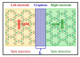
**Figure 5** Schematic illustration of a HOMF-graphene-HOMF spintronic device.
