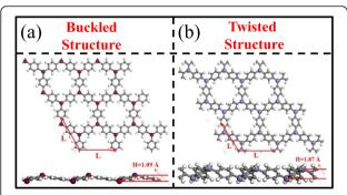
Figure 1 Two kinds of structures of triphenyl-TM lattices: buckled structure and twisted structure. (a) Top view and side view of triphenyl-Cr lattice as an example; (b) top view and side view of triphenyl-Mn lattice as an example. L is the lattice constant, H is the buckling height.
