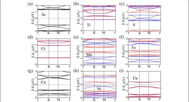
**Figure 3** Spin-polarized band structures of the triphenyl-TM lattices. (a-i) Spin-polarized band structures of the triphenyl-TM lattices from Sc to Cu. Black curves in (a) and (g) mean nonmagnetic bands; blue and red curves in other plots are the spin-up and spin-down bands, respectively. Only spin-down (red) bands are shown in (d) and (i) for AFM lattices.
