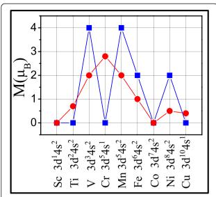
Figure 2 Magnetic moments per unit cell (blue square) and per TM atom (red circle) for different triphenyl-TM lattices.
