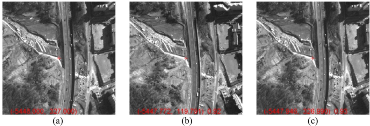
Fig. 15 An image matching result between the left and right epipolar image pair from IKONOS-2. a, b the left and the right image, respectively. c The left image which shows the reversed matching result
