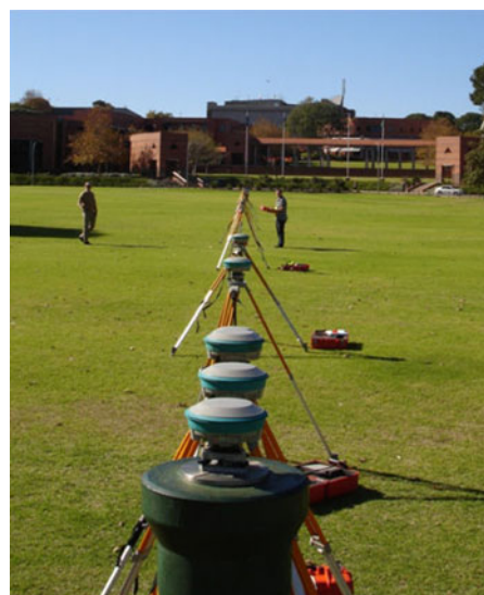
Fig. 2 Set-up of 2nd static experiment (Australia), with the five baselines of varying length
