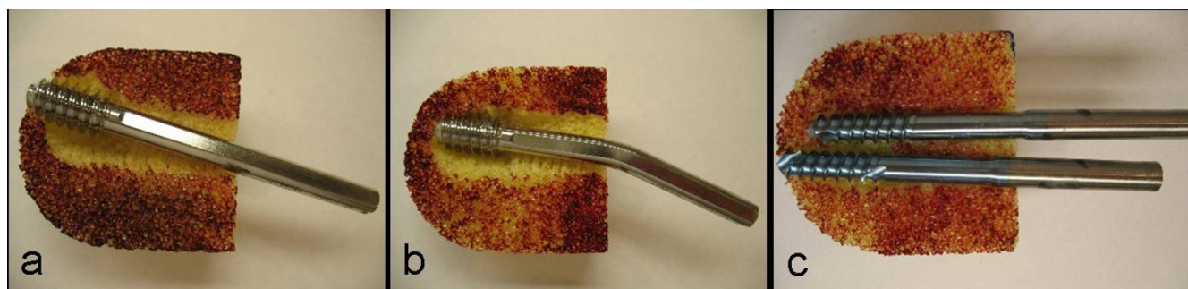
Figure 4 Lag screw failure modes: a) DHS varus collapse and subsequent cut-out failure, b) lag screw bending in absence of cut-out, and c) axial migration of distal Endovis screw, leading to cut-out despite minimal varus collapse.
