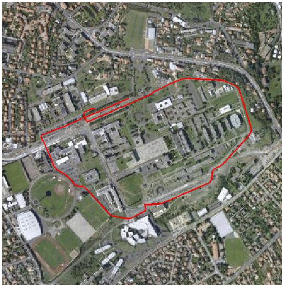
Figure 11 Robot's ground truth trajectory (using D-Gps) during the velocity estimation experiment (2 km).
