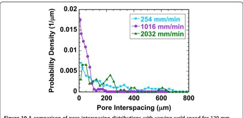
Figure 10 A comparison of pore-interspacing distributions with varying weld speed for 120 mm focal length at 600 W. At the high (2032 mm $\times$  min $^{-1}$ ) and low (254 mm $\times$  min $^{-1}$ ) speeds, several pores are found at large distances from one another, while at the medium (1016 mm $\times$  min $^{-1}$ ), weld speed pores are clustered relatively closely.
