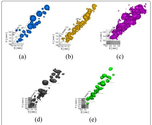
Figure 2 3D reconstructions of weld porosity produced at a focal length of 120 mm under a delivered power of 600 W and travel speeds of (a) 254 mm  $\times$  min<sup>-1</sup>, (b) 508 mm  $\times$  min<sup>-1</sup>, (c) 1016 mm  $\times$  min<sup>-1</sup>, (d) 1524 mm  $\times$  min<sup>-1</sup>, (e) 2032 mm  $\times$  min<sup>-1</sup>, illustrating decreasing average pore size at higher travel speeds and highest shape complexity occurring at 1016 mm  $\times$  min<sup>-1</sup>.
