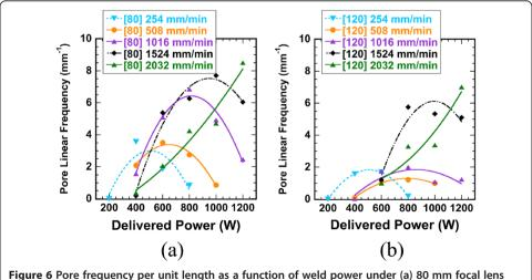
Figure 6 Pore frequency per unit length as a function of weld power under (a) 80 mm focal lens and (b) 120 mm focal lens.
