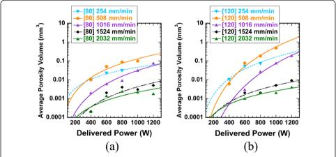
Figure 5 Average pore volume as a function of weld power under (a) 80 mm focal lens and (b) 120 mm focal lens showing an increase in pore volume with weld power and decreases in travel speed.
