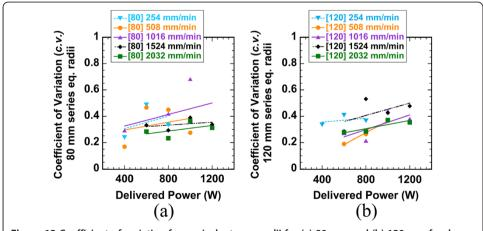
Figure 12 Coefficient of variation for equivalent pore radii for (a) 80 mm and (b) 120 mm focal distance welds indicating very small variability in pore size across all weld schedules examined.
