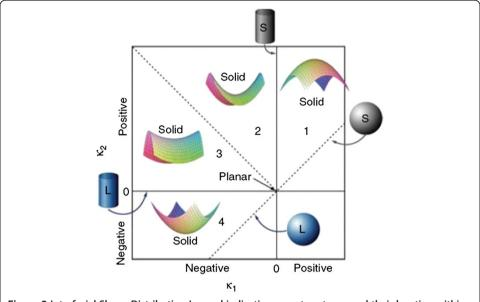
**Figure 3** Interfacial Shape Distribution Legend indicating curvature types and their location within the ISD [20,22,23]. Reprinted from Acta Materialia, Vol. 54, issue 6, D. Kammer, P. Voorhees, "The Morphological Evolution of Dendritic Microstructures During Coarsening", pp. 1549–1558, (2006), with permission from Elsevier.
