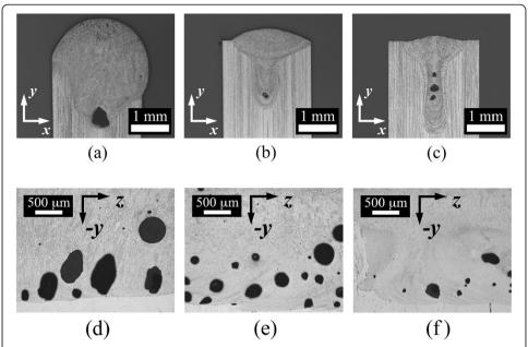
Figure 1 Transverse (a-c) and longitudinal (d-f) micrographs of welds produced under a power of 1200 W at (a, d) 1016 mm  $\times$  min<sup>-1</sup>, (b, e) 1524 mm  $\times$  min<sup>-1</sup> and (c, e) 2032 mm  $\times$  min<sup>-1</sup>. Transverse cross-sections show keyhole weld geometries including porosity and surrounding base metal, and longitudinal micrographs taken along welding direction further indicate scale of porosity present.
