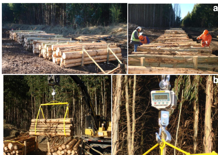
Fig. 1 a Layout of log piles of E. globulus and E. nitens set for the air-drying experiment. Piles were about 1.4 m wide, 1 m tall and 244 cm or 350 cm in length. Trials were started in winter, spring and summer with three factors: species ( E. globulus , E. nitens ), debarking (with bark, without bark) and length (2.44 m, 3.50 m). b Detail of pile-weighing procedure and the dynamometer
