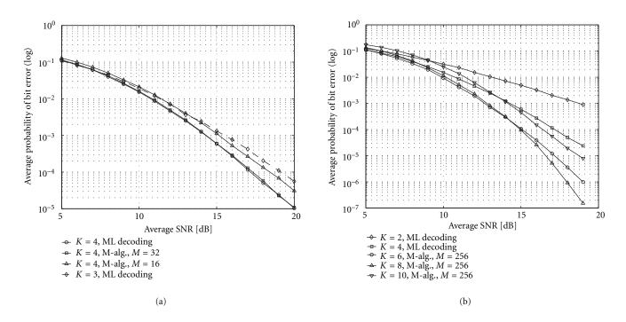
FIGURE 8: Simulation results IV. (a) Four antennas, suboptimal decoding, (b) ST codes for QPSK modulation.
