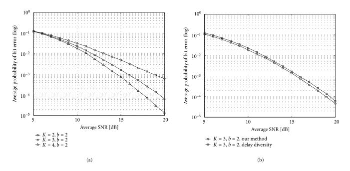
FIGURE 5: Simulation results I. (a) Delay diversity with QPSK, (b) three transmit antennas with QPSK.
