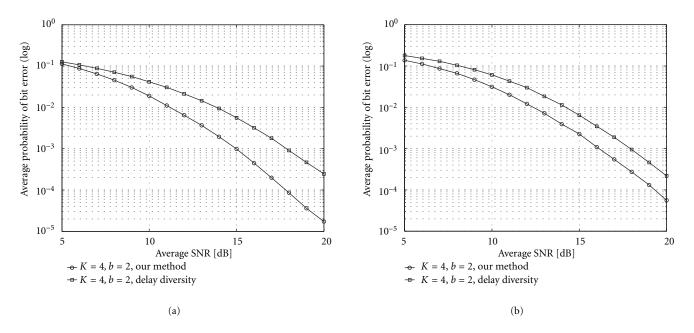
FIGURE 7: Simulation results III. (a) Four transmit antennas with asymmetric QPSK, (b) four transmit antennas with 4ASK.
