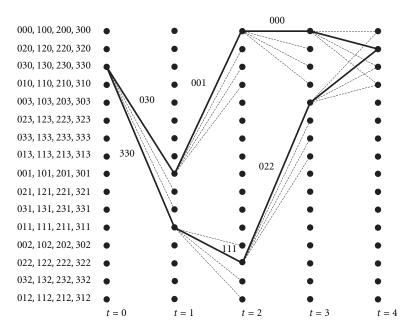
FIGURE 1: Example ST code for three antennas, QPSK.
