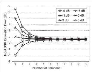
Figure 3 Input SNR estimation error (in dB) with respect to number of iterations used in iterative estimation.
