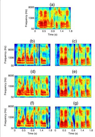
Figure 1 Illustration of separating two male utterances in cochannel conditions. (a) Cochleagram of the cochannel speech with an input SNR of –9 dB. (b) Cochleagram of clean target. (c) Cochleagram of clean interferer. (d) Cochleagram of initially segregated target. (e) Cochleagram of initially segregated interferer. (f) Cochleagram of segregated target after iterative estimation. (g) Cochleagram of segregated interferer after iterative estimation.
