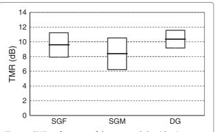
**Figure 6** TMR performance of the proposed algorithm in different kinds of cochannel speech with 0-dB input TMR.
