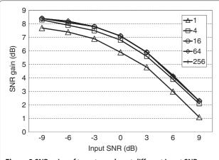
Figure 2 SNR gains of target speaker at different input SNR conditions with beam width varying from 1 to 256.
