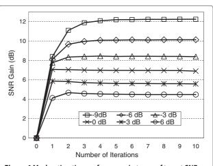
**Figure 4** Mask estimation performance in terms of target SNR gain as a function of number of iterations.
