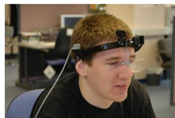
Figure 1: Magnetic Tracker device
