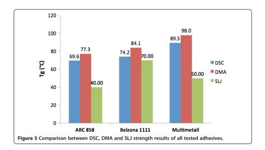
that the service temperature of polymer composites when used as adhesives cannot be determined only by thermal analyses since the joint resistance is not solely dependent of the adhesive temperature resistance, but is also outcome of the adhesion forces between the adhesive and the substrate, this last a function of temperature as well.
