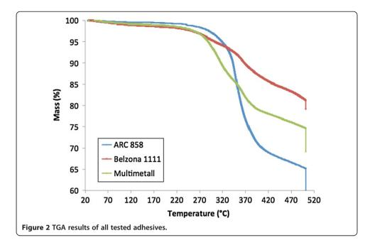
fillers and the mass fraction of filler added to each material. Figure 2 displays the TGA results of all tested adhesives.
