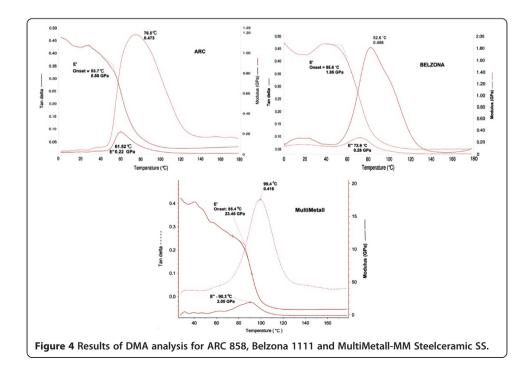
It is possible to notice a difference of 10 percent, approximately, between the Tg values measured by DSC and DMA for each of the ARC 858 samples and Belzona 1111. Barral et al. [14] assigns the highest value for the analyses by high-DMA measurements to the differences in the frequency for each analysis. This is because the dynamic analysis by DMA (heating rate ones), have a residual heat of reaction, thus masking the real value of the glass transition temperature.
