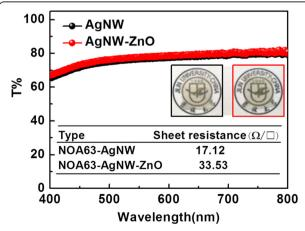
Figure 5 Light transmittance of AgNW anode on photopolymer substrate before and after growing ZnO.
