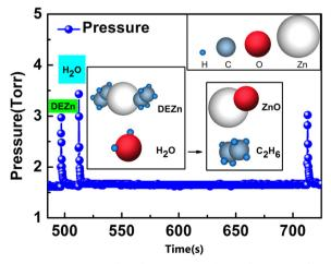
Figure 2 Precursor pulse of  $Zn(C_2H_5)_2$  and  $H_2O$  during ZnO film deposition in ALD process.
