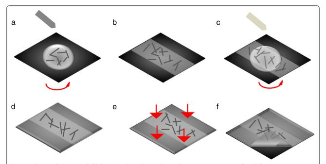
**Figure 1 Ultrasmooth AgNW anode fabricated on photopolymer substrate by spin-coating process and peel-off process. (a)** AgNW suspension drop down on Si substrate and spin-coating at 8,000 rpm for 30 s; **(b)** dry in ambient environment room temperature; **(c)** NOA63 drop down and spin-coating for first spinning at 300 rpm for 15 s, second spinning at 800 rpm for 15 s; **(d)** after spin-coating; **(e)** UV curing at 300 W (370 nm) for 4 min; **(f)** peel-off process.
