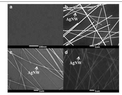
**Figure 4** The top surface of SEM images. (a) ZnO grown on Si substrate; (b) AgNWs on Si substrate; (c) AgNWs after being transferred and embedded in the photopolymer substrate via spin-coating process and peel off; (d) ZnO-AgNWs in the photopolymer substrate.
