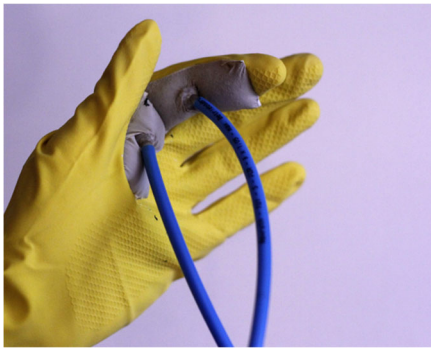
Fig. 13 Prototype of jamming pads
