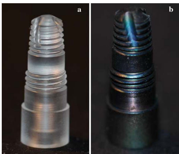
Fig. 1 Macroscopic pictures of a non-coated PMMA implant (A) titanium-coated PMMA implant (B). The titanium coating has a shiny, gray-black appearance
