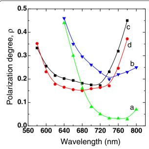
**Fig. 3** Spectra of the polarization degree for porous of nc-Si-SiO<sub>x</sub> sample, which were treated in HF solution for 5 (a, b) and 17 (c, d) min. The polarization of the exciting light was oriented parallel to the projection of the inclined SiO<sub>x</sub> nanocolumns on the sample plane (b, c) and in perpendicular direction (a, d)
