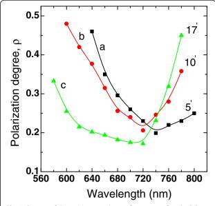
**Fig. 2** Spectra of the polarization degree for porous of  $nc-Si-SiO_x$  sample, in which PL spectra are shown in Fig. 1. The numbers near the curves indicate the time of treatment in HF solution in minutes
