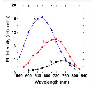
**Fig. 1** PL spectra of porous nc-Si–SiO<sub>x</sub> sample annealed in vacuum, then treated in 0.5 % HF solution for 5 (a), 10 (b), and 17 (c) min. The spectra were measured for parallel orientation of the analyzer to polarization of the exciting radiation, and polarization of the exciting light is oriented parallel to the projection of the inclined SiO<sub>x</sub> nanocolumns on the sample plane
