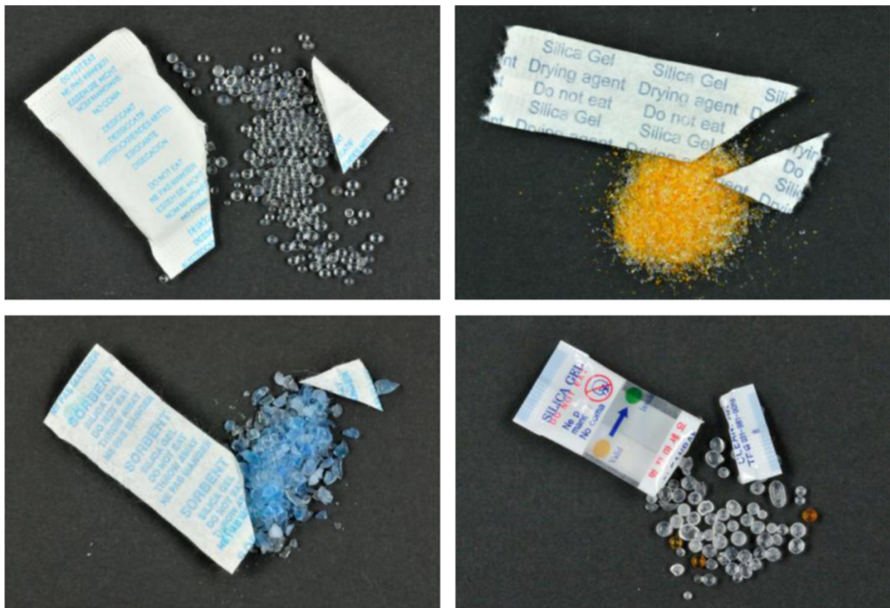
Figure 4 Different types of silica gel. Upper left: non-indicating silica gel, transparent or opaque beads. Upper right: self-indicating silica gel, methyl violet as the humidity (colour) indicator. Lower left: self-indicating silica gel, cobalt dichloride. Lower right: partial-indicating silica gel: a majority of non-indicating beads with a few indicator beads.
