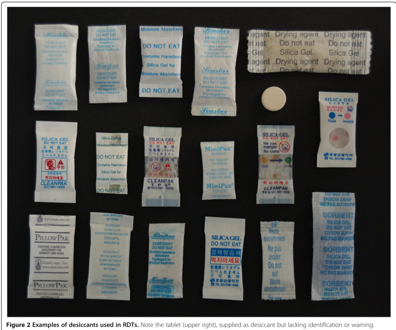
Figure 2 Examples of desiccants used in RDTs. Note the tablet (upper right), supplied as desiccant but lacking identification or warning.
