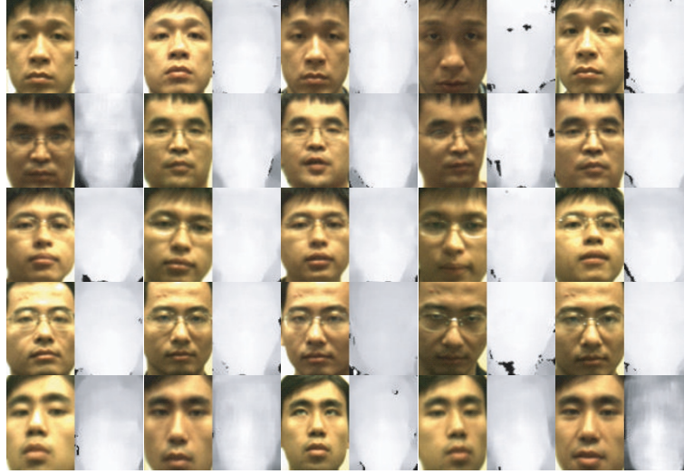
FIGURE 4: Normalized appearance and disparity images captured by the Mega-D stereo head.
